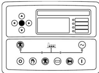
DS7320. It has a digital LCD screen, which provides easy reading of the information regarding the engine, alternator, mains and load.
