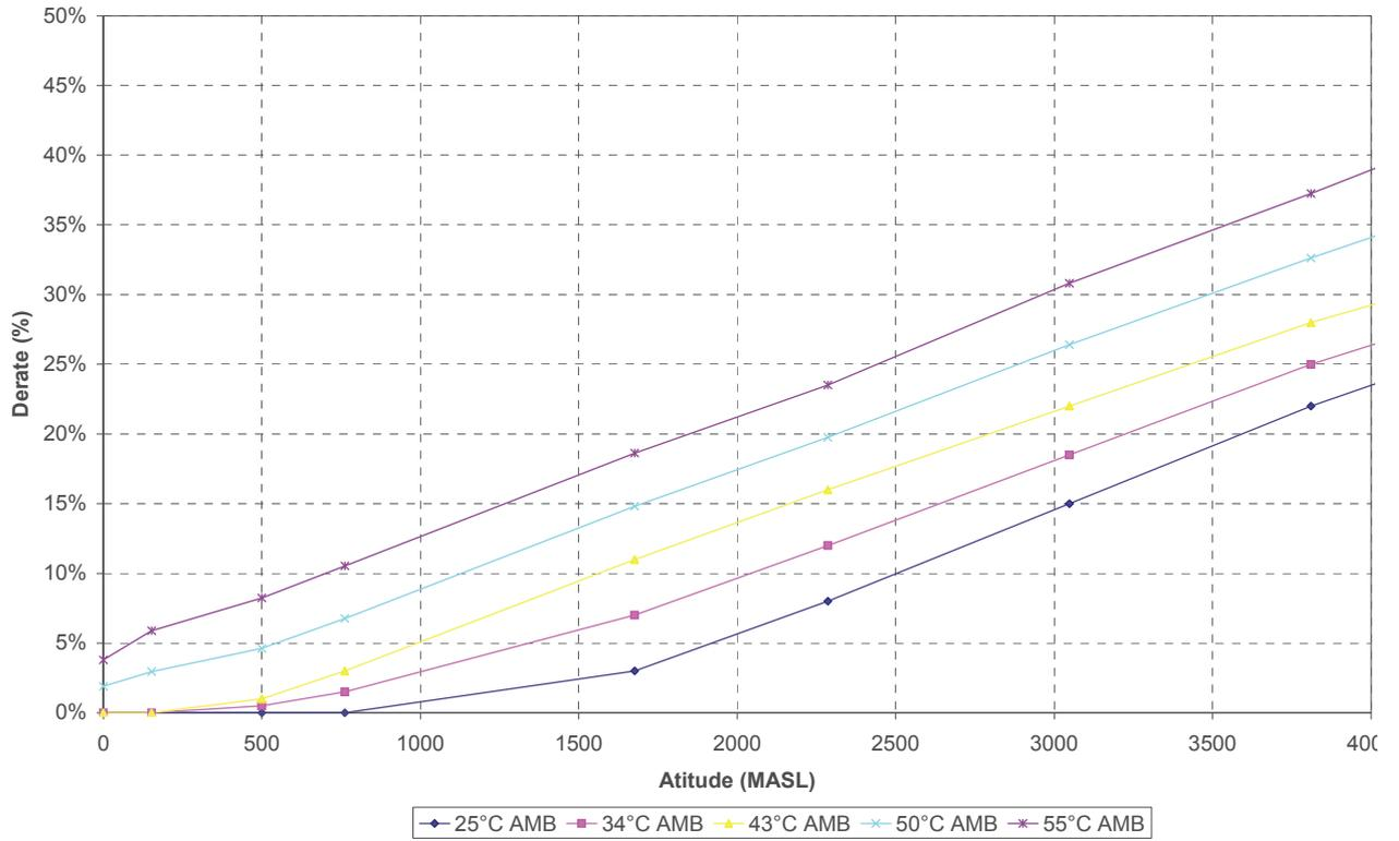
**Note:** Ambient temperature at air cleaner inlet.
